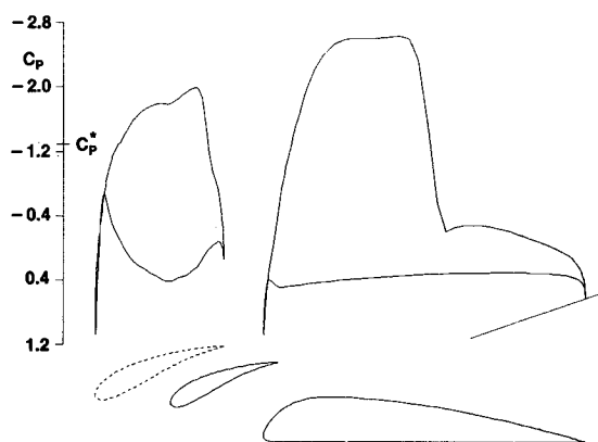
Fig. 11 Surface pressure distribution computed on Clark-Y airfoil with Maxwell slat, M_\infty = 0.600 , \alpha = 4.0 deg.
