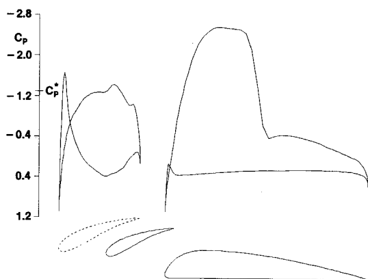
Fig. 10 Surface pressure distribution computed on Clark-Y airfoil with Maxwell slat, M_\infty = 0.600 , \alpha = 2.5 deg.
